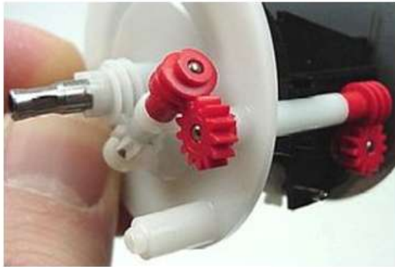
Fig 3. Worm gear positioning in odometer
